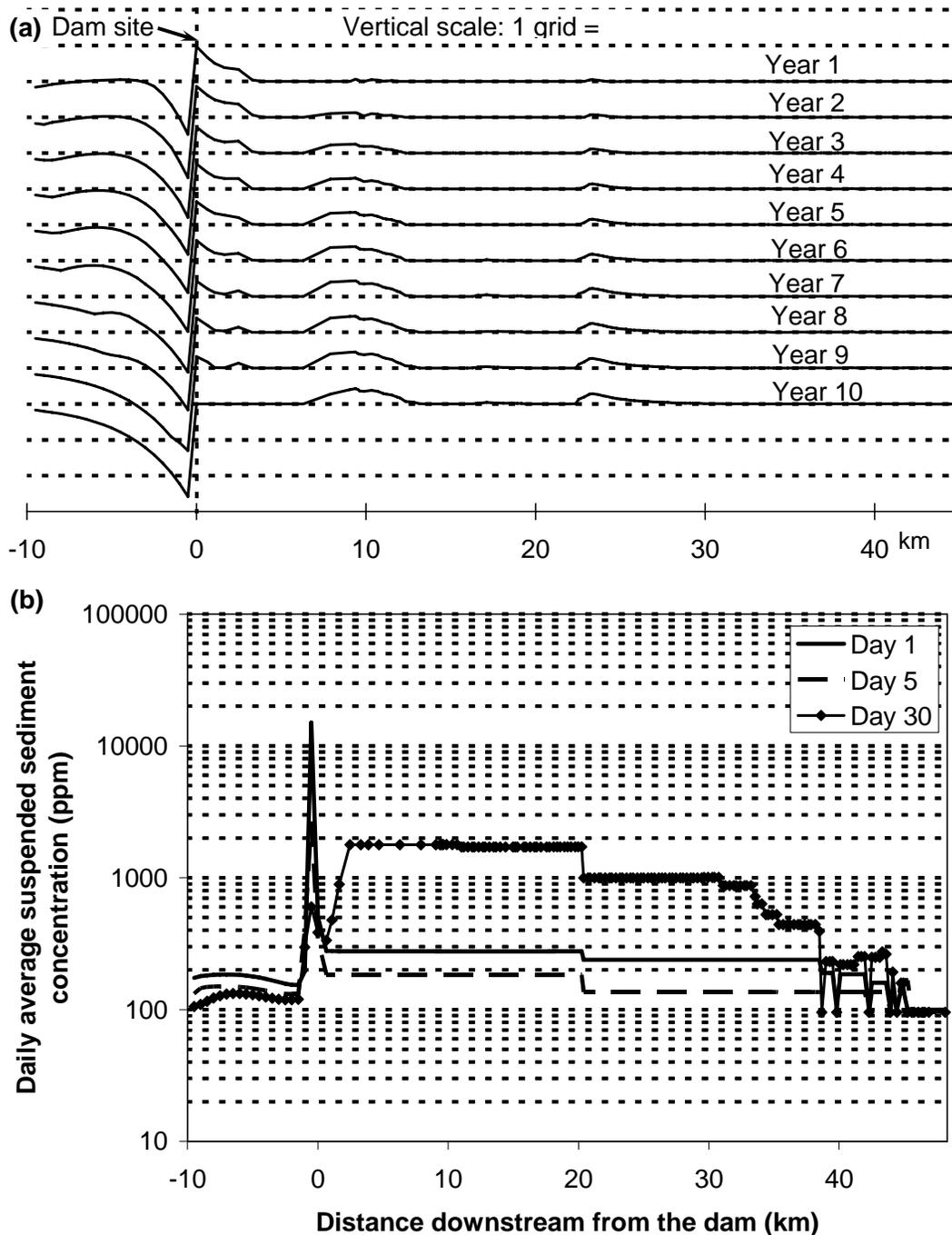
**Figure 9.** *DREAM-2* simulation results for the case the reservoir deposit is composed of mixtures of gravel/pebble and sand under the blow-and-go scenario: (a) cumulative aggradation/degradation following dam removal; and (b) weekly maximum daily average suspended sediment concentration following dam removal.
