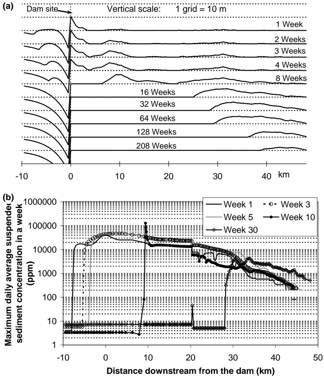
**Figure 7.** *DREAM-1* simulation results for the case the reservoir deposit is composed of 0.5-mm sand under the blow-and-go scenario: (a) cumulative aggradation/degradation following dam removal; and (b) weekly maximum daily average suspended sediment concentration following dam removal.
