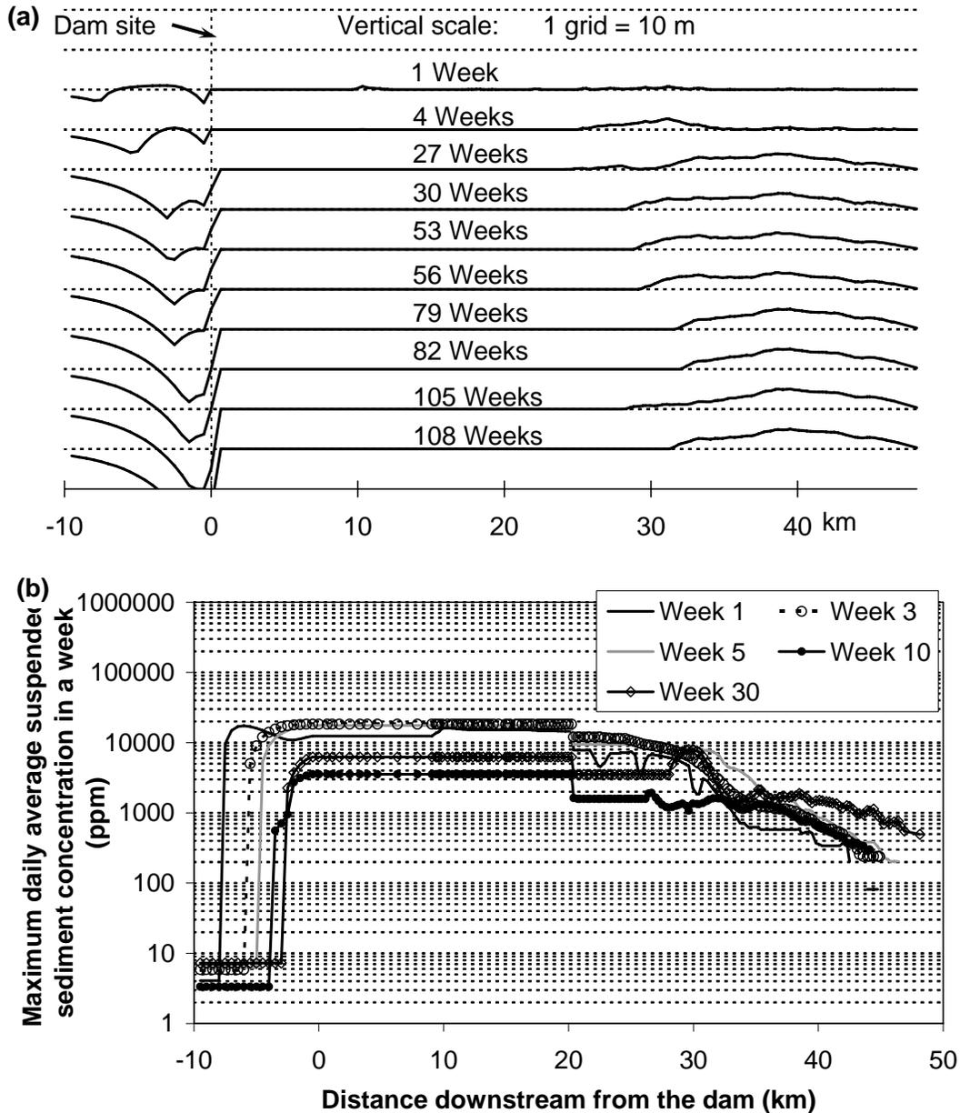
**Figure 8.** *DREAM-1* simulation results for the case the reservoir deposit is composed of 0.5-mm sand under the staged removal scenario: (a) cumulative aggradation/degradation following dam removal; and (b) weekly maximum daily average suspended sediment concentration following dam removal.
