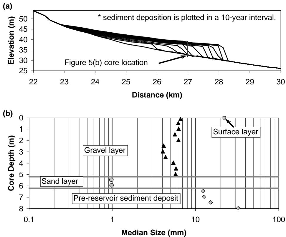
**Figure 5.** Simulated sediment deposition process in a reservoir, indicating delta formation and migration (a) and stratification of sediment deposition (b). The hypothetical dam is located at 50 km (outside of Figure 5a) with a crest elevation of 40 m.
