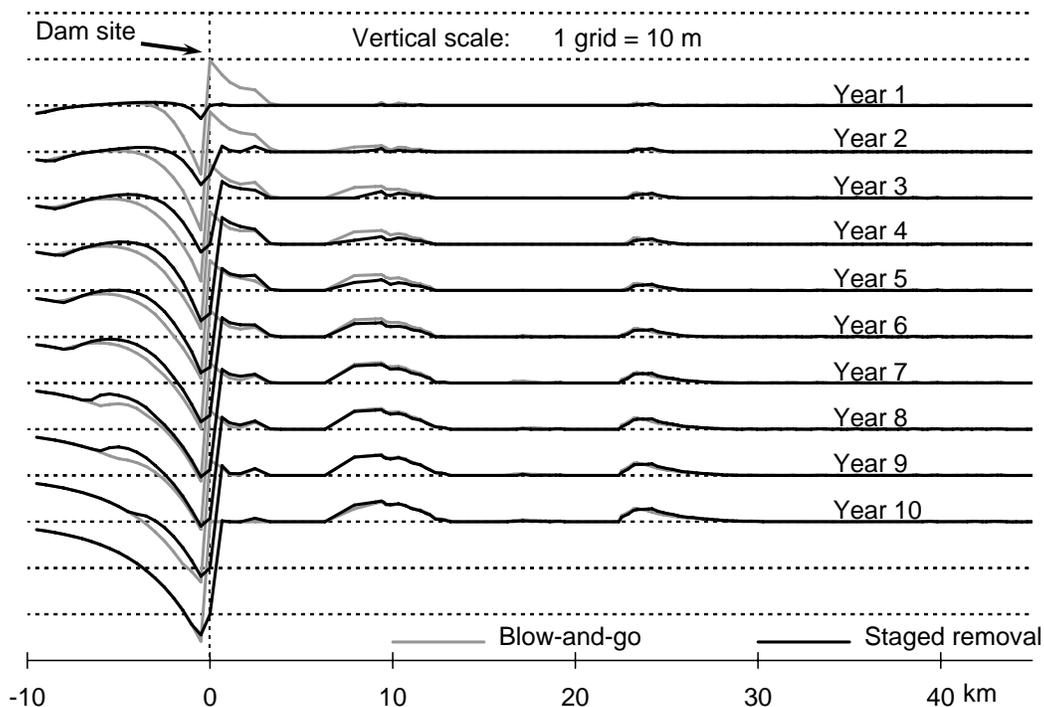
**Figure 10.** DREAM-2 simulation results for the case the reservoir deposit is composed of a mixture of gravel/pebble and sand under the staged removal scenario: cumulative aggradation/degradation following dam removal. Results for the blow-and-go scenario are also presented for comparison purposes.
