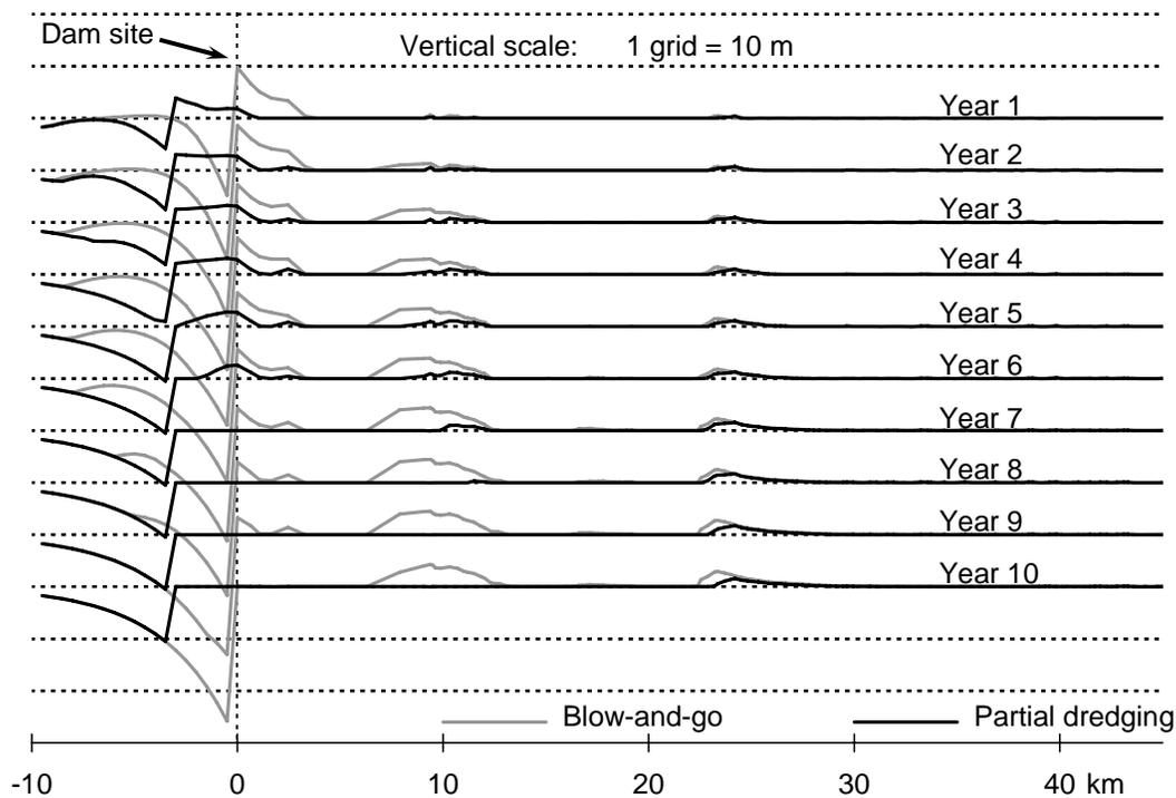
**Figure 11.** *DREAM-2* simulation results for the case the reservoir deposit is composed of a mixture of gravel/pebble and sand with partial dredging prior to dam removal: cumulative aggradation/degradation following dam removal. Results for the blow-and-go scenario are also presented for comparison purposes.
