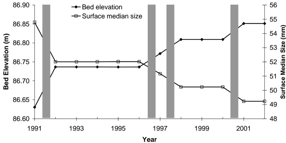
**Figure 2.** Simulated reach-average bed elevation and surface median size at a location (~1.0 km on Figure 1) where gravel was augmented on four occasions (indicated by bars in the figure).
