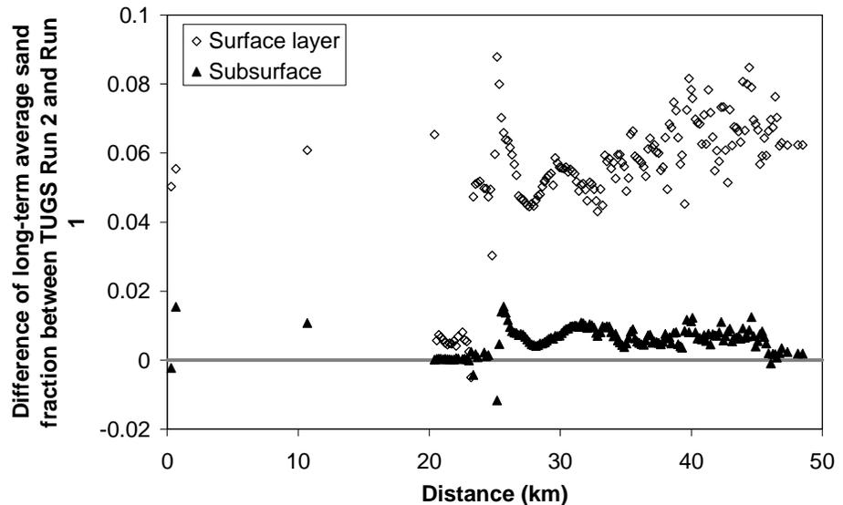
**Figure 4.** Simulated increase in sand fraction in a 50-km river reach if sediment supply is doubled. Areas without data points (*i.e.*, upstream of 20 km) are bedrock reaches where there were no sediment deposits during the period of simulation.
